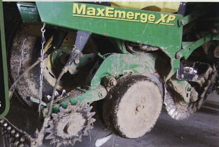
NO-TILL SETUP. Row cleaners, fluted no-till coulters, seed firmers, spiked closing wheels and leveling tines make up the no-till planting package on the row units of Howard Buffett's John Deere planter.
